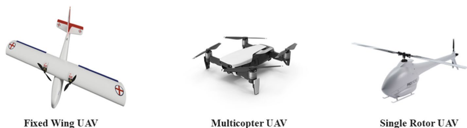
Fig. 4 Common types of unmanned aerial vehicles (UAVs) employed in fire management
